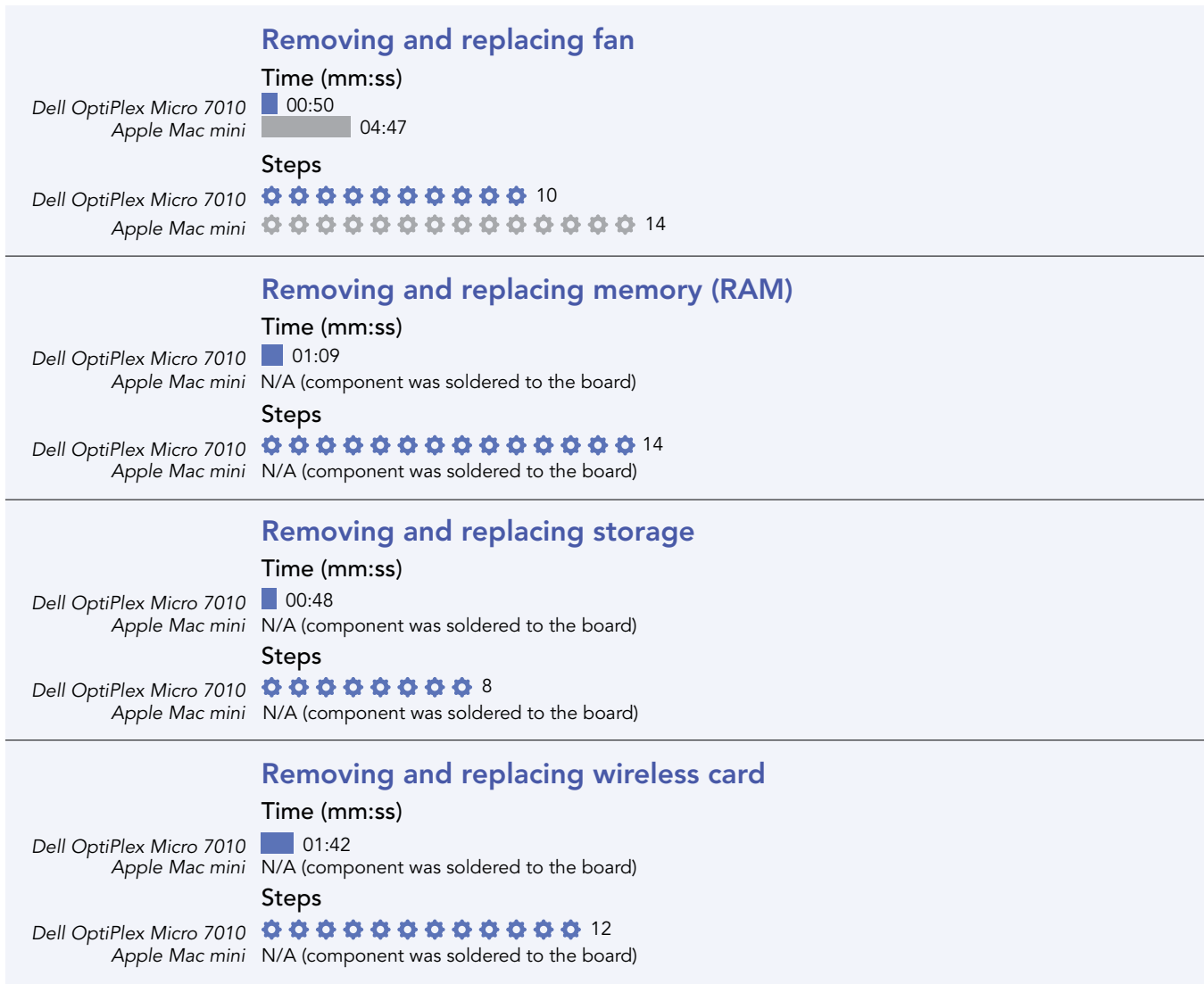
Figure 3: Time and steps required to remove and replace four components from the Dell OptiPlex Micro 7010 and Apple Mac mini. Lower is better. Source: Principled Technologies.
