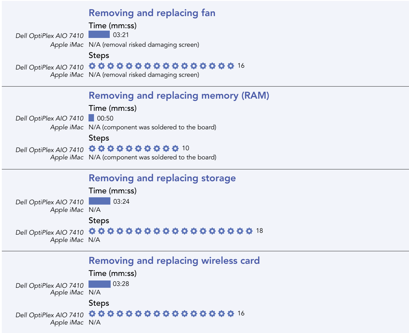
Figure 4: Time and steps required to remove and replace four components from the Dell OptiPlex AIO 7410 and Apple iMac. Lower is better. Source: Principled Technologies.
