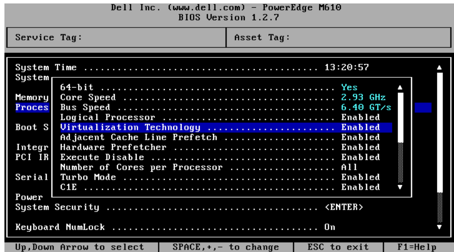
Figure 4. Example BIOS configuration for the Dell PowerEdge M610 showing virtualization technology enabled.
