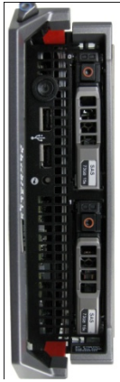
Dell PowerEdge M610 blade server featuring Intel Xeon Processor 5500 series
