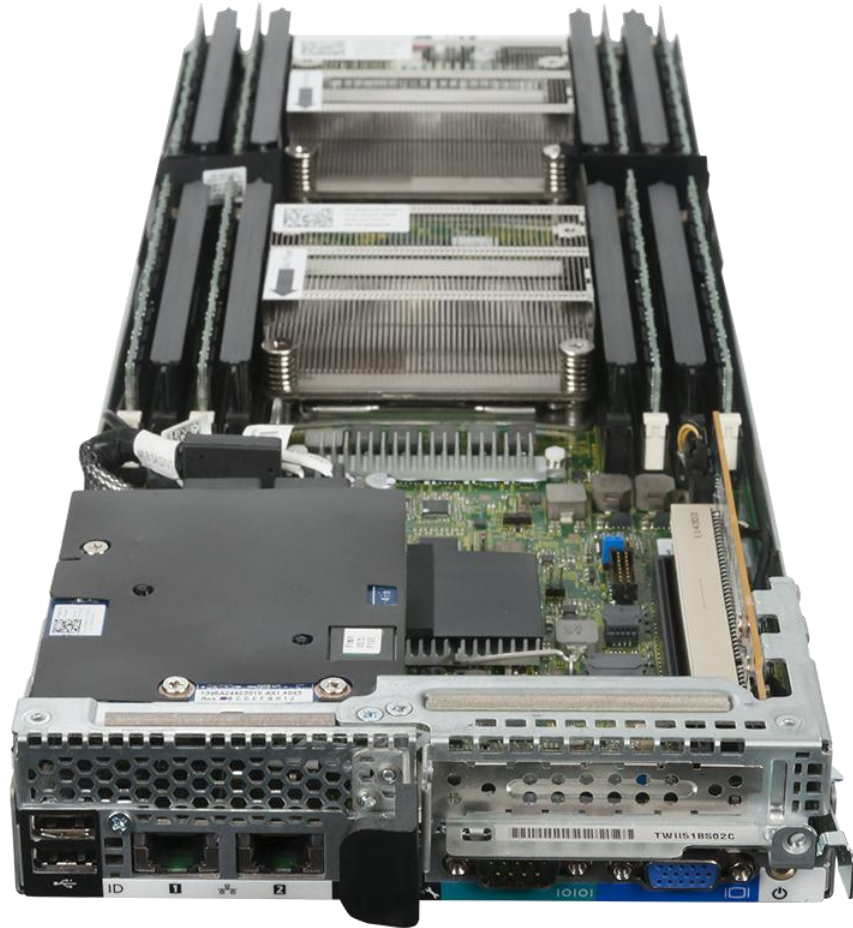
Figure 1: 1U server node of the Dell PowerEdge C6220 with the LSI SAS2008 mezzanine card.
