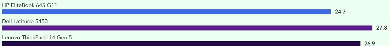
Figure 13: Median acoustic results while the PCs were plugged in and running the Cinebench 2024 benchmark for 30 minutes. Lower decibels are better. Source: Principled Technologies.
