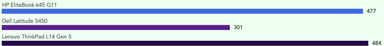
Figure 12: Median performance scores while the PCs were plugged in and running the Cinebench 2024 benchmark for 30 minutes. Higher performance scores are better. Source: Principled Technologies.
