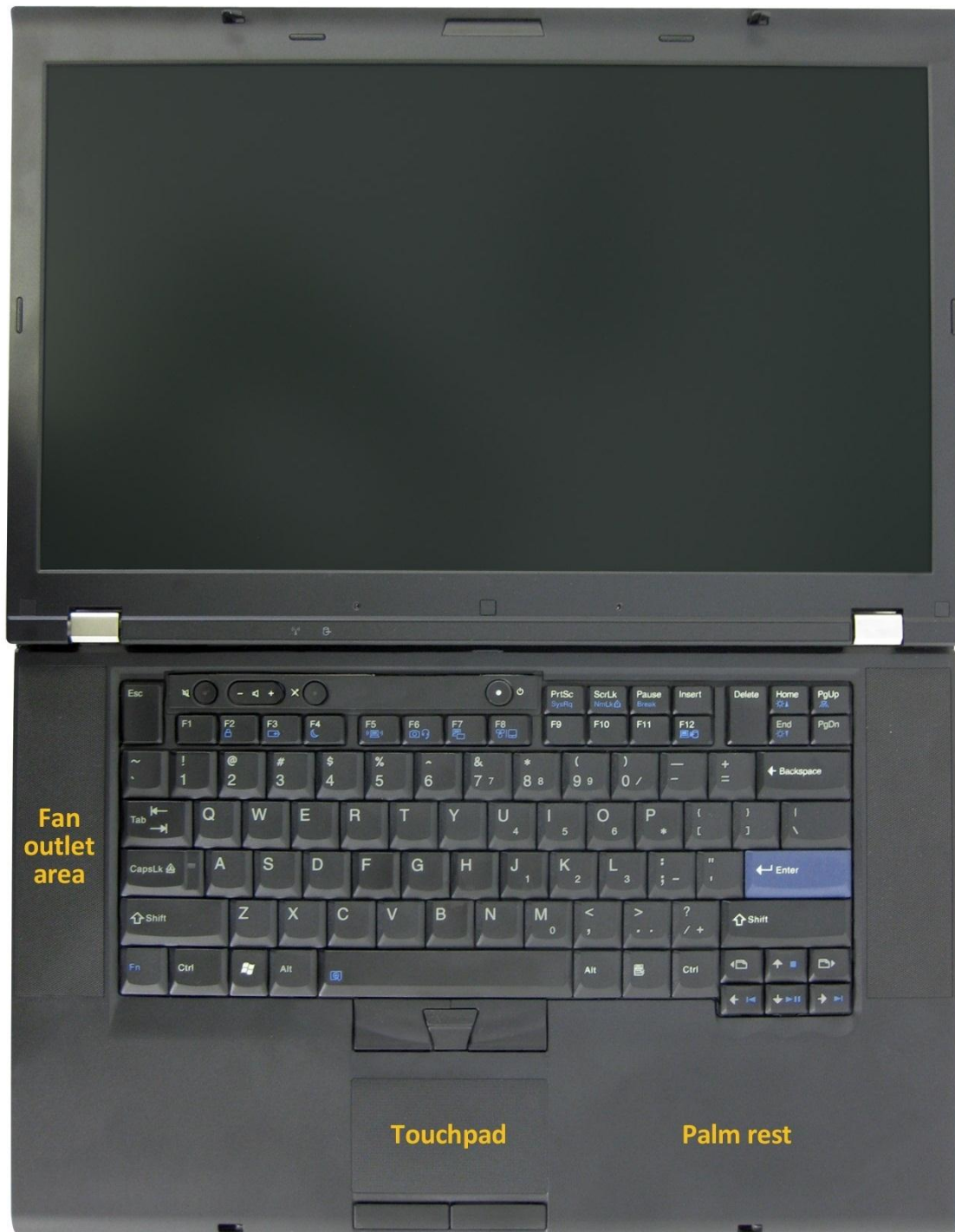
Figure 10: Yellow text indicates the areas where we measured temperature.
