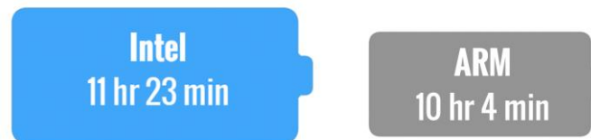
Figure 1: The amount of the time the two Chromebooks lasted unplugged while browsing the Internet.
