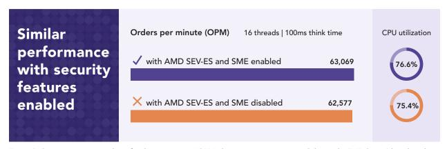
Figure 2: **Center:** Average number of orders per minute (OPM) the environment processed during the DVD Store 3 benchmark workload, using settings of 16 threads and 100ms think time. Higher is better. **Right:** Average CPU utilization of the environment during the DVD Store 3 workload. Our virtualized environment consisted of a Dell PowerEdge R7625 server powered by AMD EPYC 9274F processors. The server ran Red Hat Enterprise Linux 8. Source: Principled Technologies.
