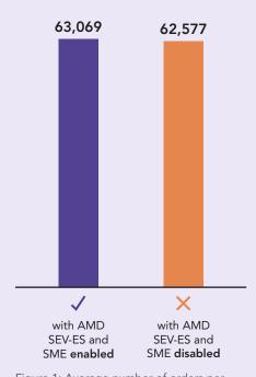
Figure 1: Average number of orders per minute (OPM) the environment processed during the DVD Store 3 benchmark workload, using settings of 16 threads and 100ms think time. Higher is better.
