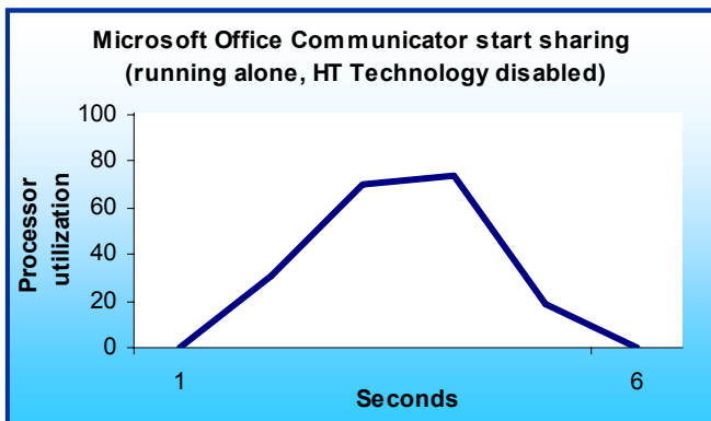
Figure 23: System processor utilization of the Microsoft Office Communicator start sharing foreground task running alone on the Intel Pentium 4 630 Processor-based PC with HT Technology disabled.
