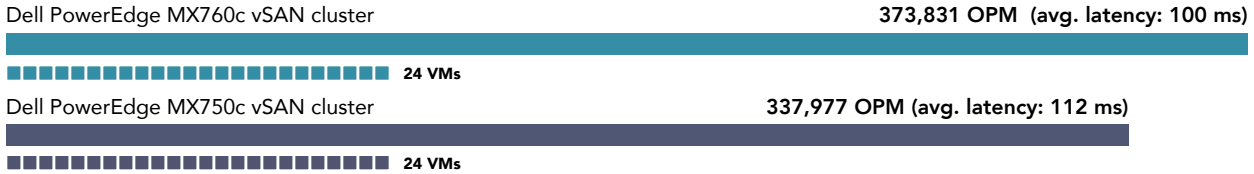
Figure 1: Total orders per minute the two clusters achieved with 24 VMs. Higher OPM and lower latency are better. Source: Principled Technologies.
