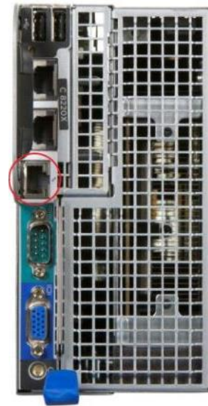
Figure 8: Management port on compute sled.
