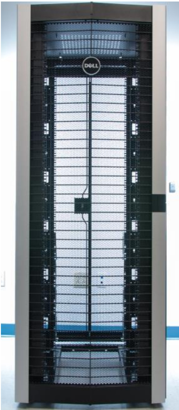
Figure 1: Dell PowerEdge 4220W rack.
