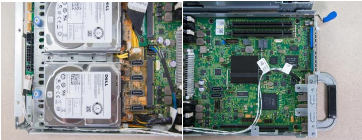
Figure 5: BMC cable installation.
