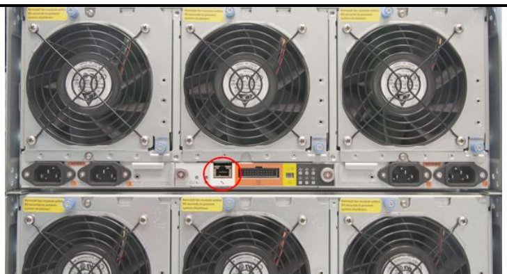
Figure 7: Rear BMC management port on chassis.
